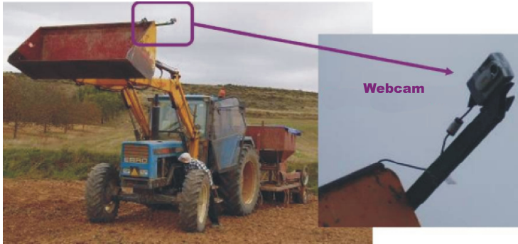
Fig. 7. Installation of the webcam in the tractor
