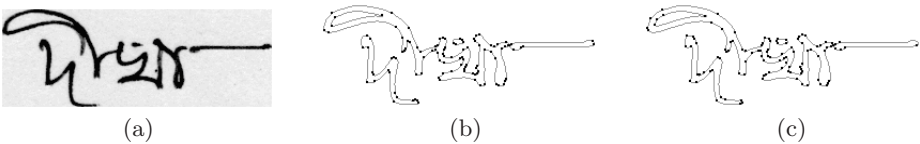
Fig. 4. (a) Original image (b) Feature points extracted in anticlockwise direction (c) Feature points extracted in clockwise direction
