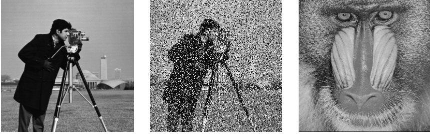
Fig. 1. The MSE does not always correspond to human evaluation of image comparison: left = original cameraman image, middle = cameraman image with 35% salt & pepper noise (MSE w.r.t. left image = 7071), right = monkey image (MSE w.r.t. left image = 5061)
