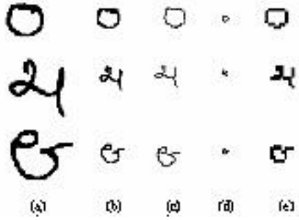
Fig. 3. (a) Original Image, (b) Normalized image, (c) Thinned image,(d) Reduced image, (e) Enlarged view of reduced image
